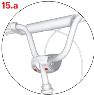
15.a Installing the protective covers (One, Two)
